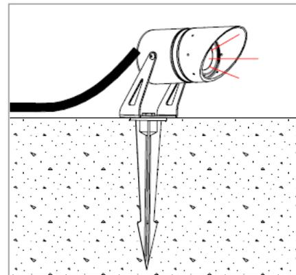
PER INSTALLAZIONI AD ALTEZZE OLTRE I 5 METRI UTILIZZARE FISCHER IDONEI IN FUNZIONE DEL PESO DEL PRODOTTO FOR INSTALLATION OVER 5 METRES HEIGHT, USE SUITABLE FISHER ACCORDING TO THE WEIGHT OF THE PRODUCT
